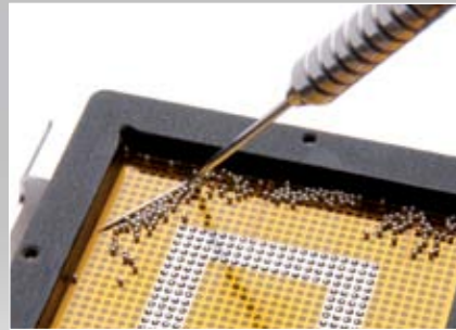
Distributing balls in modified Universal Eco-Mask.
