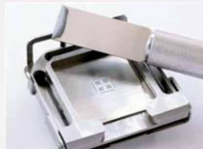
Application of solder paste with the squeegee.
